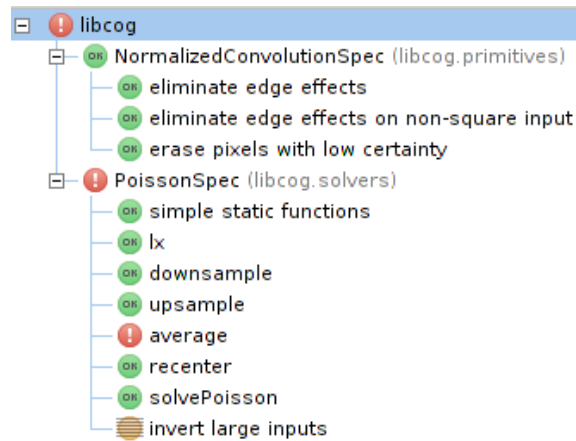
Figure 3·2: Sample test report for a library of visual algorithms. The implementation of normalized convolution exercised by the NormalizedConvolutionSpec test suite passed all of its tests, as indicated by the green “OK” icon next to the test suite and each test contained in the suite. The PoissonSpec suite failed one behavioral test (“average”), indicated by the red error icon. PoissonSpec also contains one test without a complete implementation (“invert large inputs”), indicated by the yellow icon. Without a complete test implementation, the test runner cannot determine if the test passed or failed and thus marks it as pending. The test runner generated this report in under a minute on a standard workstation and with no human intervention.
